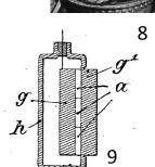
**Dec 1917**: Mosaic of thin quartz slices mounted between  $\lambda/4$  steel plates. Resonant at 40 kHz
