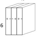
**June 1917:** 3 quartz slices bonded together resonate at 60kHz
