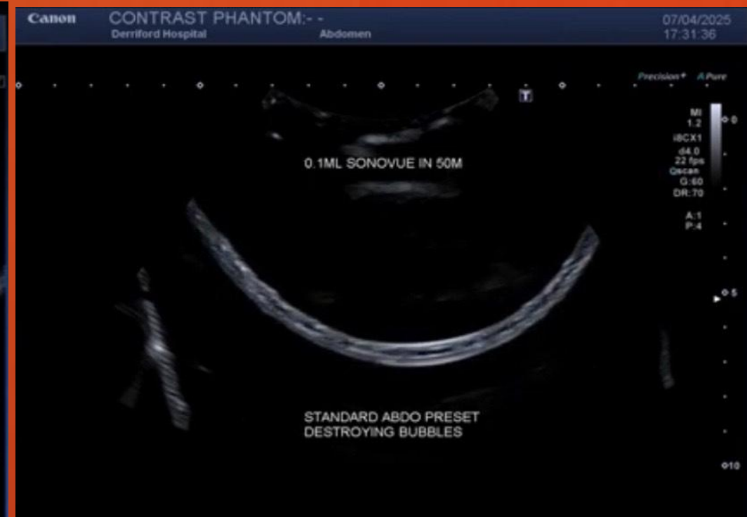
Image 12.: Using a mechanical index (MI) of 1.2 with the standard abdominal preset resulted in destruction of microbubble contrast agents.
