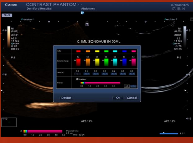
Images 13-15.: Parametric Calc: Parametric Microflow Imaging (Hanlon, 2025) Colour-coded parametric mapping visualises microbubble flow and arrival time, providing a temporal map of contrast movement within the imaging field.
