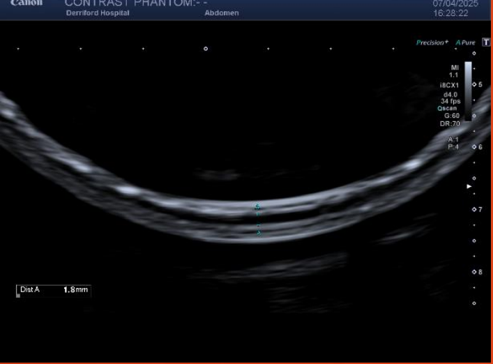
Image 2.: The lumen of the tube was measured using B-mode imaging.
