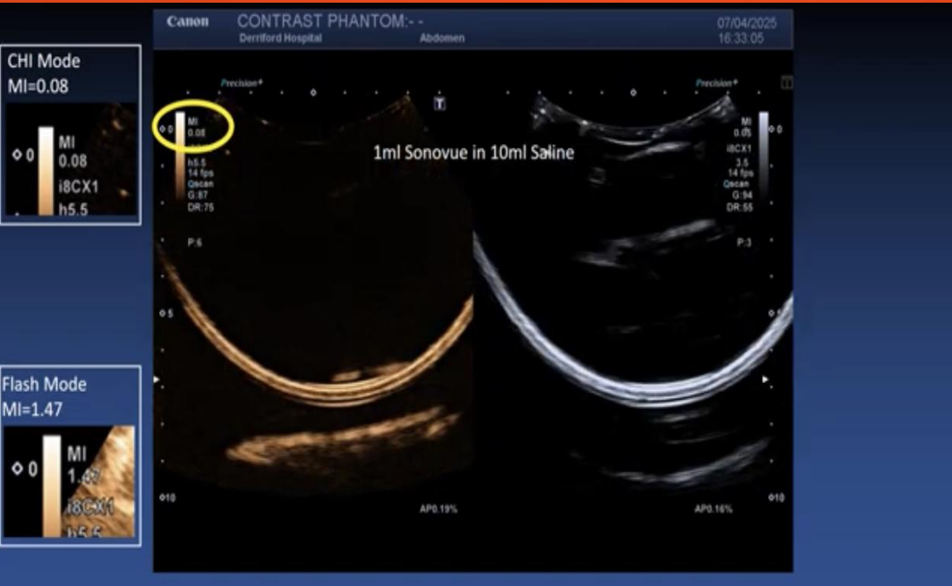
Image 8.: Activating the Flash button resulted in complete microbubble destruction within the lumen of the Foley catheter.
