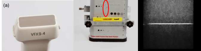
Figure 1 (a) example probe used for the tests (b) probe mounted on the jig. The position of the pins used in the test is highlighted. (c) example image obtained at one probe position during an experiment.
