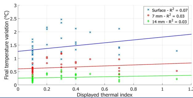
Goodness of fit decreases with depth using infrared data and increases when output power is used, suggesting that absorption plays a more important role deeper in tissue.
